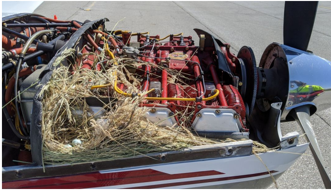
ENGINE PLUGS PREVENT BIRD NEST FOD. Piper Saratoga Engine Cowling Bird's Nest Zenith 701 Engine Inlet Plugs
