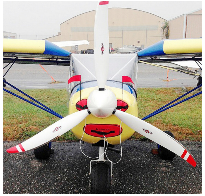
ENGINE PLUGS PREVENT BIRD NEST FOD. Piper Saratoga Engine Cowling Bird's Nest Zenith 701 Engine Inlet Plugs
