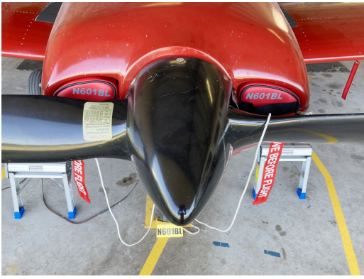
Zenith CH 601 XLB Engine Inlet Plugs ENGINE PLUGS PREVENT BIRD NEST FOD. Piper Saratoga Engine Cowling Bird's Nest
