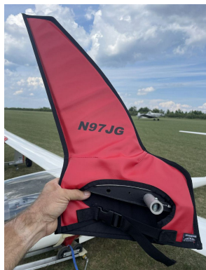
Schempp-Hirth Ventus-2B winglet/wingtip pads
