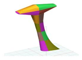
Autogyro Calidus Rotor Mast Cover, 3D model
