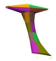
Autogyro Calidus Rotor Mast Cover, 3D model
