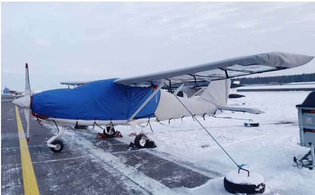
Tecnam P2010 Wing, Empennage & Prop Covers
