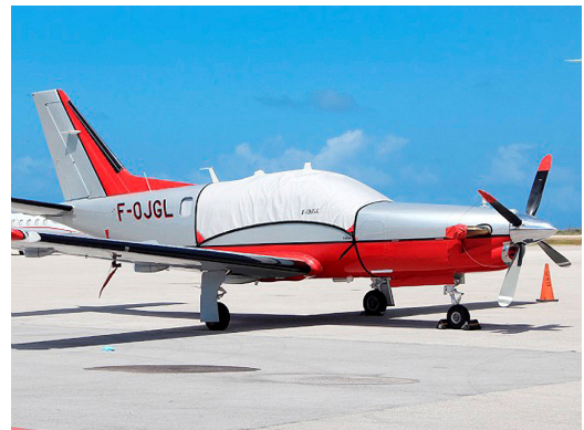
TBM Canopy Cover, Prop Tie/Exhaust Covers
