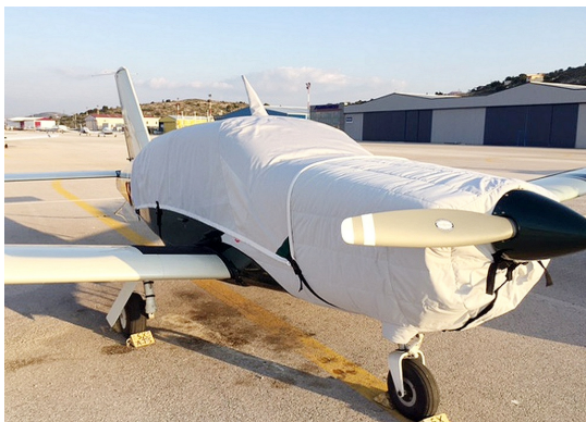
Socata TB-20 Canopy Cover, Insulated Engine Cover
