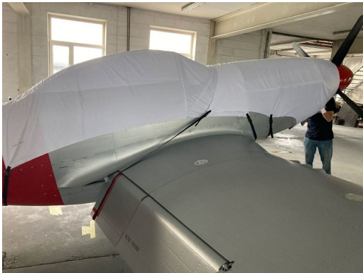
Scalewings SW-51 Mustang Canopy & Engine Covers, test fit covers
