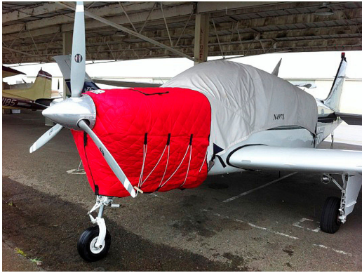
Beech Bonanza Insulated Engine Cover, fully enclosed
