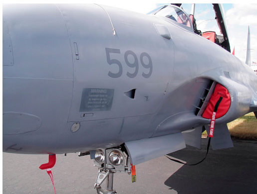
Engine Inlet Plugs and Pitot Cover
