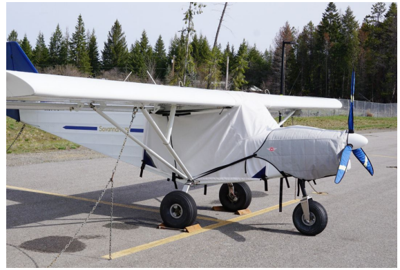
Savannah VG Canopy Cover, Insulated Engine Cover
