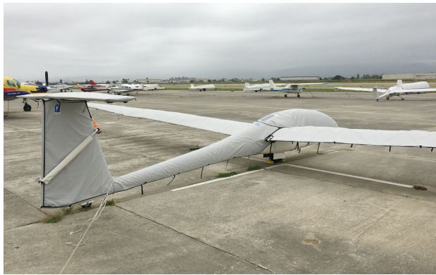
DG-505 Canopy/Nose, Wing, Empennage & Horiz. Stab. Covers
