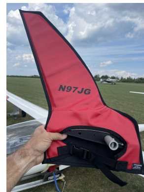
Schempp-Hirth Ventus-2B winglet/wingtip pads
