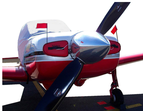
Micco SP20 Canopy Cover & Engine Inlet Plugs
