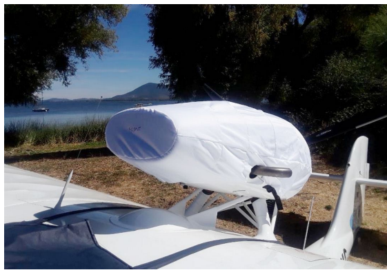
Seamax M22 Engine Cover, test fit cover
