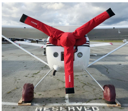
Cessna Skywagon Propellor/Spinner Cover, 3-blade type
