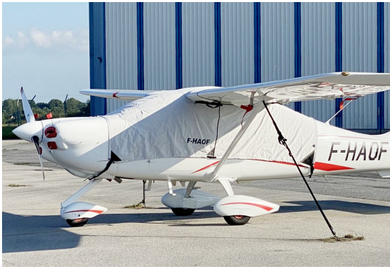
Tecnam P2010 Over-Top Canopy Cover, Engine Plugs
