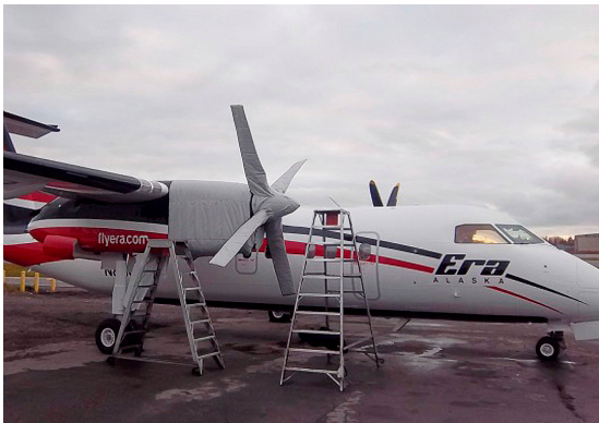
Dash 8 Insulated Engine & Prop Covers
