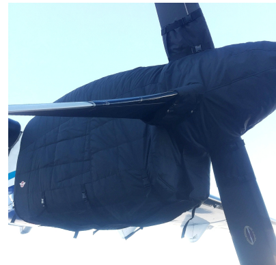
ATR-72-202 Insulated Engine & Prop Hub Covers
