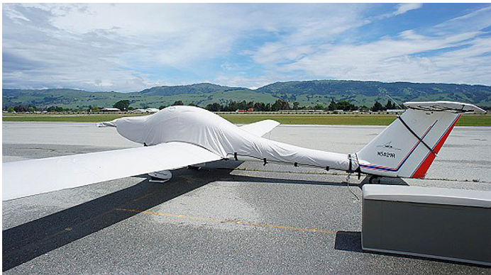
Grob 109 Canopy/Engine w/ extension to tail, Wing, Stabilizer & Prop/Spinner Covers
