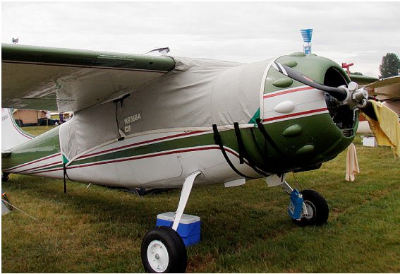
Cessna 195 Canopy Cover, extended forward and over gas caps Cessna 195 Canopy Cover, extended forward and over gas caps
