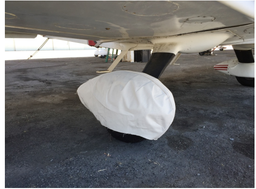
Grumman AA5 Main Wheelpant Cover, test fit
