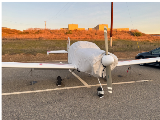
Van's Aircraft RV-6/6A Extended Canopy/Engine Cover
