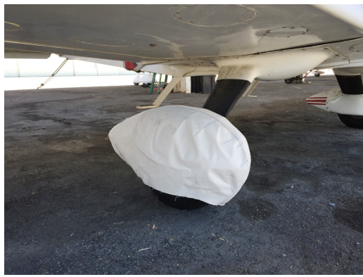
Grumman AA5 Main Wheelpant Cover, test fit
