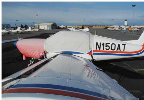
Koliber 150A Canopy Cover, Insulated Engine Cover
