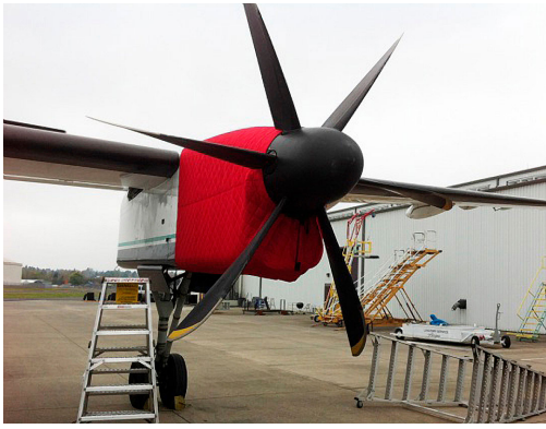
Dash 8-Q400 Insulated Engine Cover
