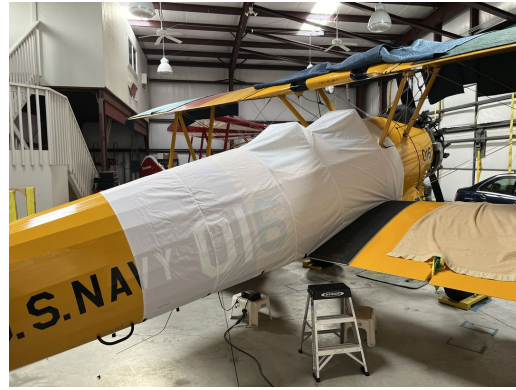
Stearman PT-13 Extended Canopy Cover, test fit cover
