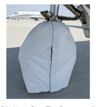
CJ1 Nose Gear Tire Cover, test fit
