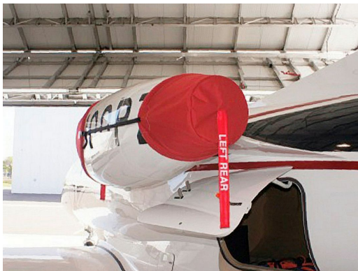
Phenom 100 Tri-fold style Engine Cover Set
