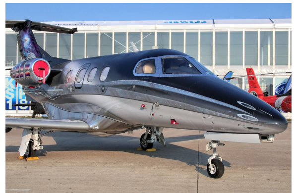
Phenom 100 Engine Inlet Plugs
