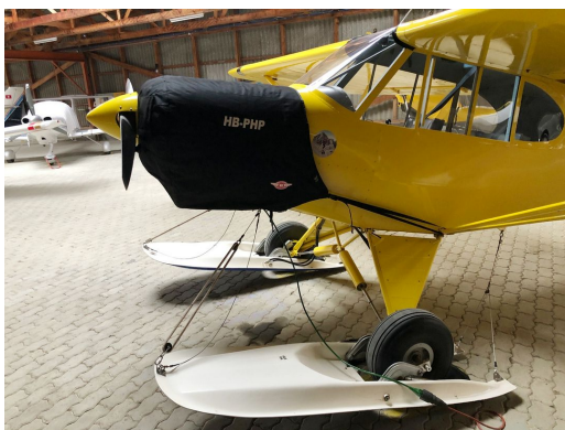
Piper PA-18 Supercub Insulated Engine Cover
