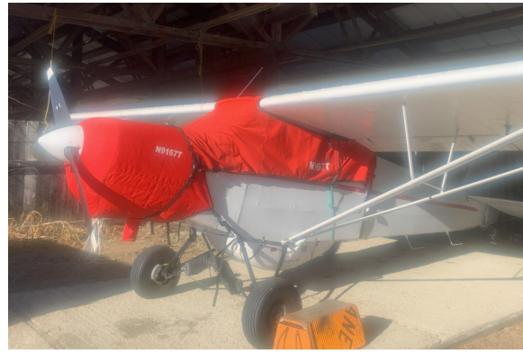
Piper PA-18 Super Cub Insulated Engine Cover, Canopy Cover
