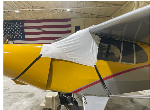
Piper J5A Windshield/Skylight Cover, test fit
