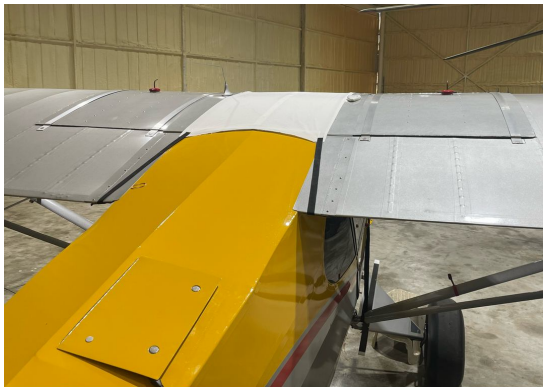
Piper J5A Windshield/Skylight Cover, test fit
