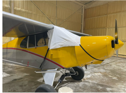
Piper J5A Windshield/Skylight Cover, test fit
