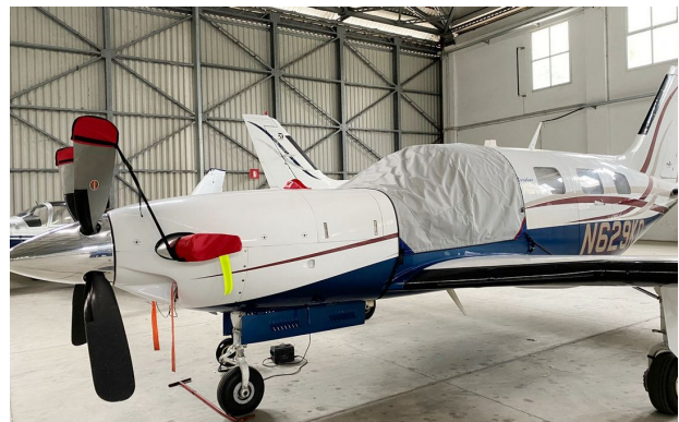
Piper PA-46-500TP Engine Cowling Top Plug
