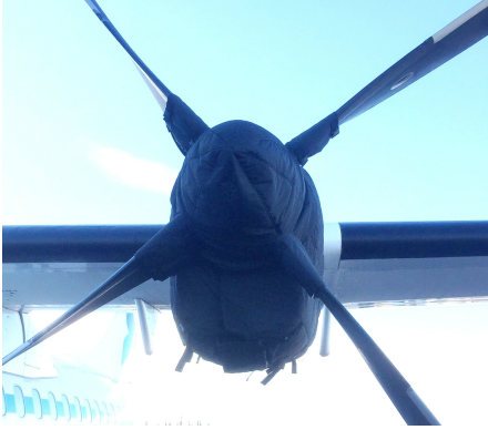
ATR-72-202 Insulated Engine & Prop Hub Covers
