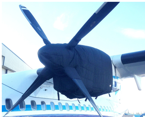
ATR-72-202 Insulated Engine & Prop Hub Covers
