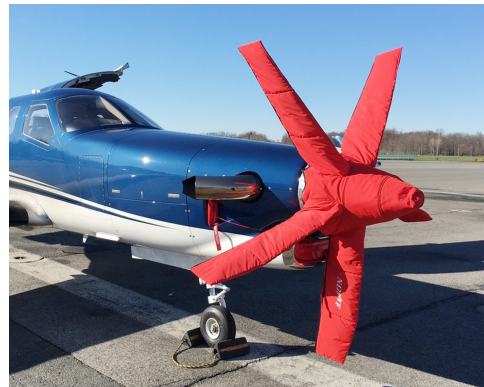
Socata TBM Insulated 5-Blade Prop/Spinner Cover
