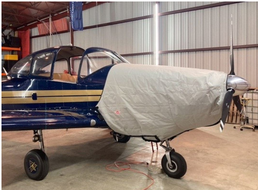
Navion Insulated Engine Cover
