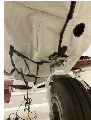
NAVION H Insulated Engine Cover
