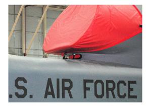
Intake Cover with small inlet plug
