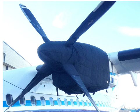
ATR-72-202 Insulated Engine & Prop Hub Covers
