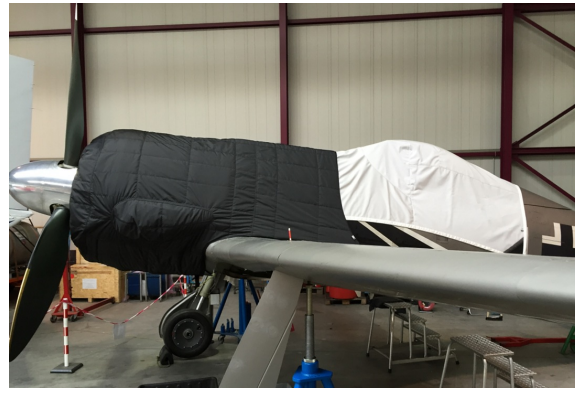
Focke Wulf 190 Canopy Cover & Insulated Engine Cover
