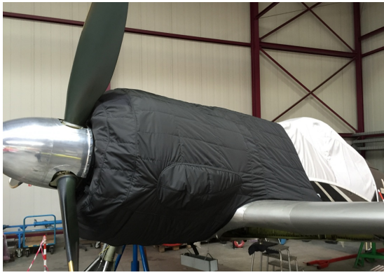
Focke Wulf 190 Canopy Cover & Insulated Engine Cover
