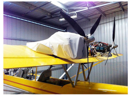
Lockwood AirCam Engine Cover (test fit cover)
