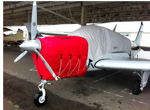
Beech Bonanza Insulated Engine Cover, fully enclosed
