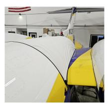
Lear 45 Empennage Saddle Cover W/ Dorsal Inlet Plug (Covers Upper Fuselage Between Pylons, Acm/Apu Area)
