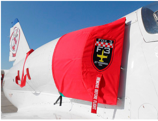
Aero L-39 Engine Cover, Snap-On Type
