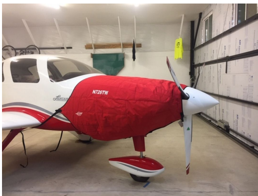
Lancair ES Insulated Engine Cover, Fully Enclosed
