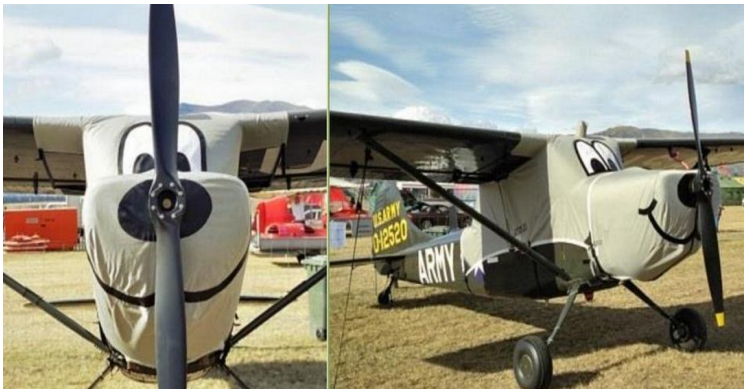
Cessna L-19 Bird Dog Canopy Cover, Engine Cover
