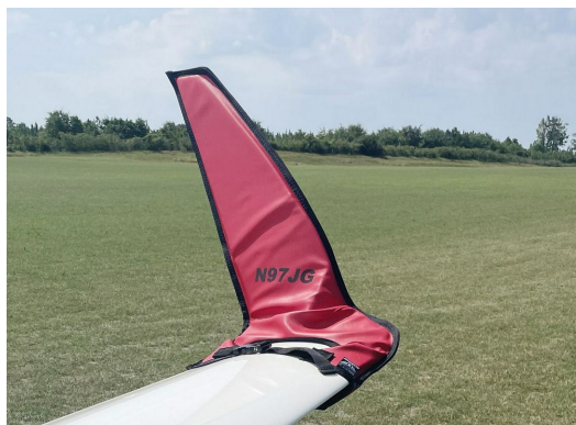
Schempp-Hirth Ventus-2B winglet/wingtip pads
