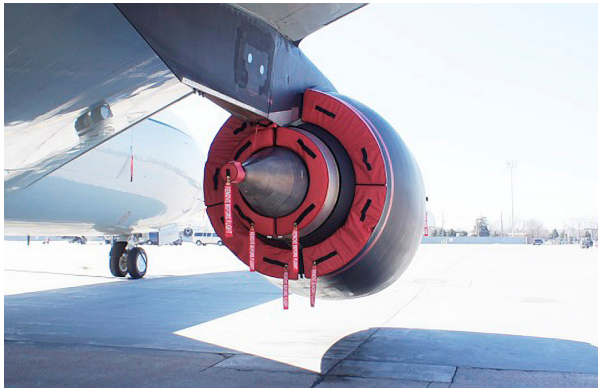
RC-135W Bypass Vent and Exhaust Plugs
