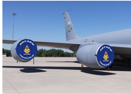
BOEING KC-135 Tambourine Type Double Fold Intake Covers, Custom Mesh Insert & IUID's with custom Imprint
