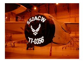
Intake/Exhaust Covers, soft type, TF-33 Engines
