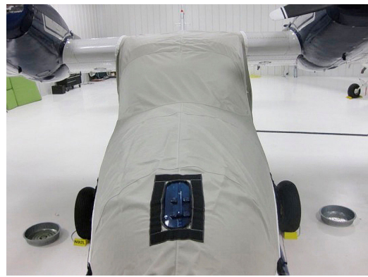
Grumman Widgeon Cockpit/Nose Cover, tie-down cleat detail
