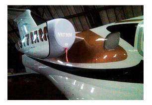
Phenom 100 Intake/Exhaust Cover, "Bikini" Type
