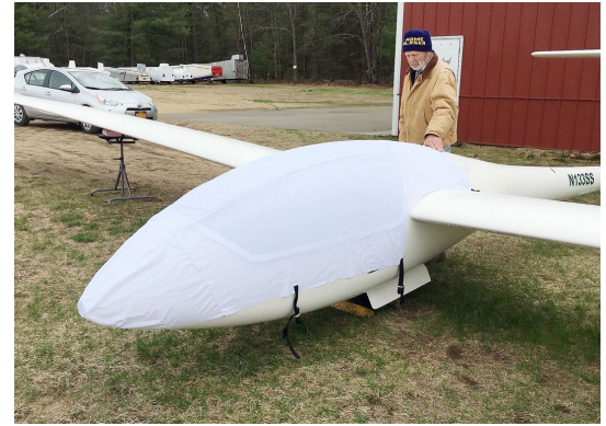
Grob 102 Astir CS Canopy/Nose Cover (test fit)
