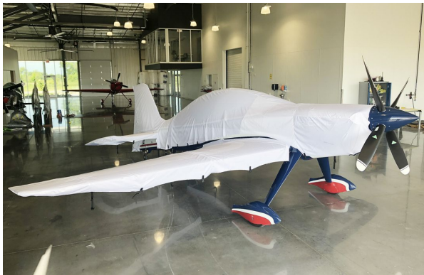
Gamebird GB-1 Extended Canopy/Engine, Wing & Empennage Covers (test fit covers)
