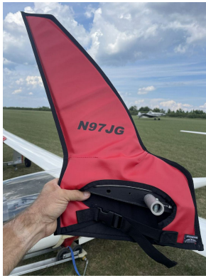
Schempp-Hirth Ventus-2B winglet/wingtip pads
