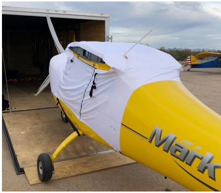
FK-Lightplanes FK-9 Canopy Cover, test fit cover
