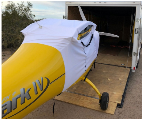
FK-Lightplanes FK-9 Canopy Cover, test fit cover
