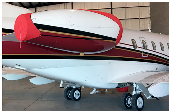
Challenger 300 Intake/Exhaust Cover Set, 3-strap type Intake/Exhaust Covers, 3-Strap Type. Successfully installed by two crew, one ladder.
